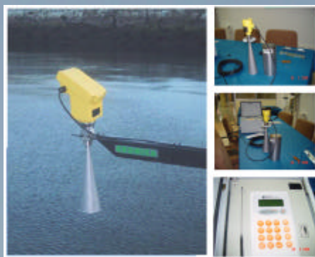
Figure 3. Radar tide gauge devices ready to be installed at L'Estartit harbour. This modern installation will work in a parallel way to the classical floating gauge active since 1992. Details of the electronics are shown in the images above and a final deployment is presented in the image below (example of the installation at Villegarda de Arosa Port, Spain). Images and deployments provided by Geonica sl, Earth Sciences.
