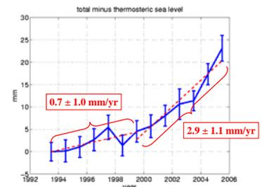
Figure 2. The difference between total and 0/750 m thermosteric sea level curves. Error bars are 95% confidence limits and reflect random error only. If there were no changes in volume average temperature at depths greater than 750 m, this curve would reflect input of freshwater into the global oceans.
