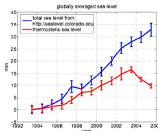
Figure 1. Globally averaged sea level. The blue curve shows total sea level based on TOPEX/Poseidon and Jason data. The red curve shows 0/750 m thermosteric sea level based on in situ profile data. Error bars are 95% confidence limits and reflect random error only.
